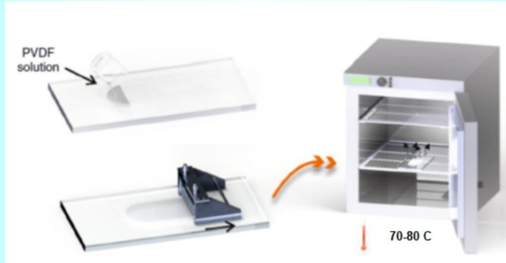
Final solutions were spread on a clean glass substrate using a coating blade with fixed distance between substrate. We use special template with fixed thickness for coating which were bonded on glass substrate. The solvent were evaporated by heating the composites in an oven at 75 °C for 15 min.
