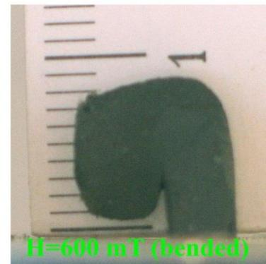
Residual deformation of a composite in a homogeneous magnetic field after mechanical deformation
